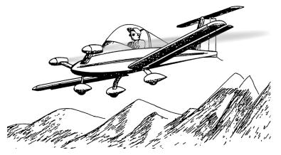
rectangular box with a streamlined canopy on top. The wing skins consist of a single standard sheet (1m x 2m) of Aluminium wrapped around the ribs and simply glued in place.
