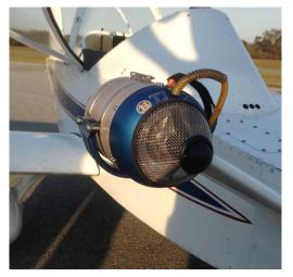
A booster with break-in clutch enabling starting of this engine from the cockpit net is located at the compressor section.
