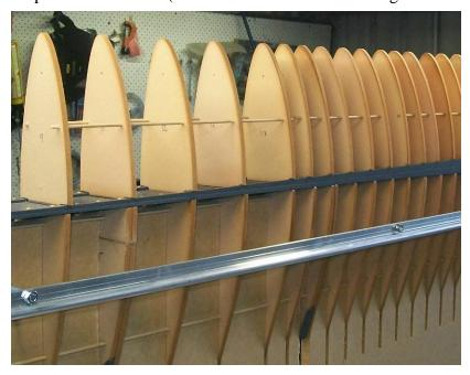
Divinycell product was substituted where required). The ribs are glued to the spar with epoxy and covered by a skin of Alclad. The result are wing surfaces smooth and free of rivets rivaling the best composite fiber lay-up construction.
