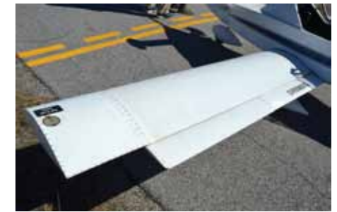
'Flaperons' combine flap and aileron function in one surface, operated through a clever mixer box
