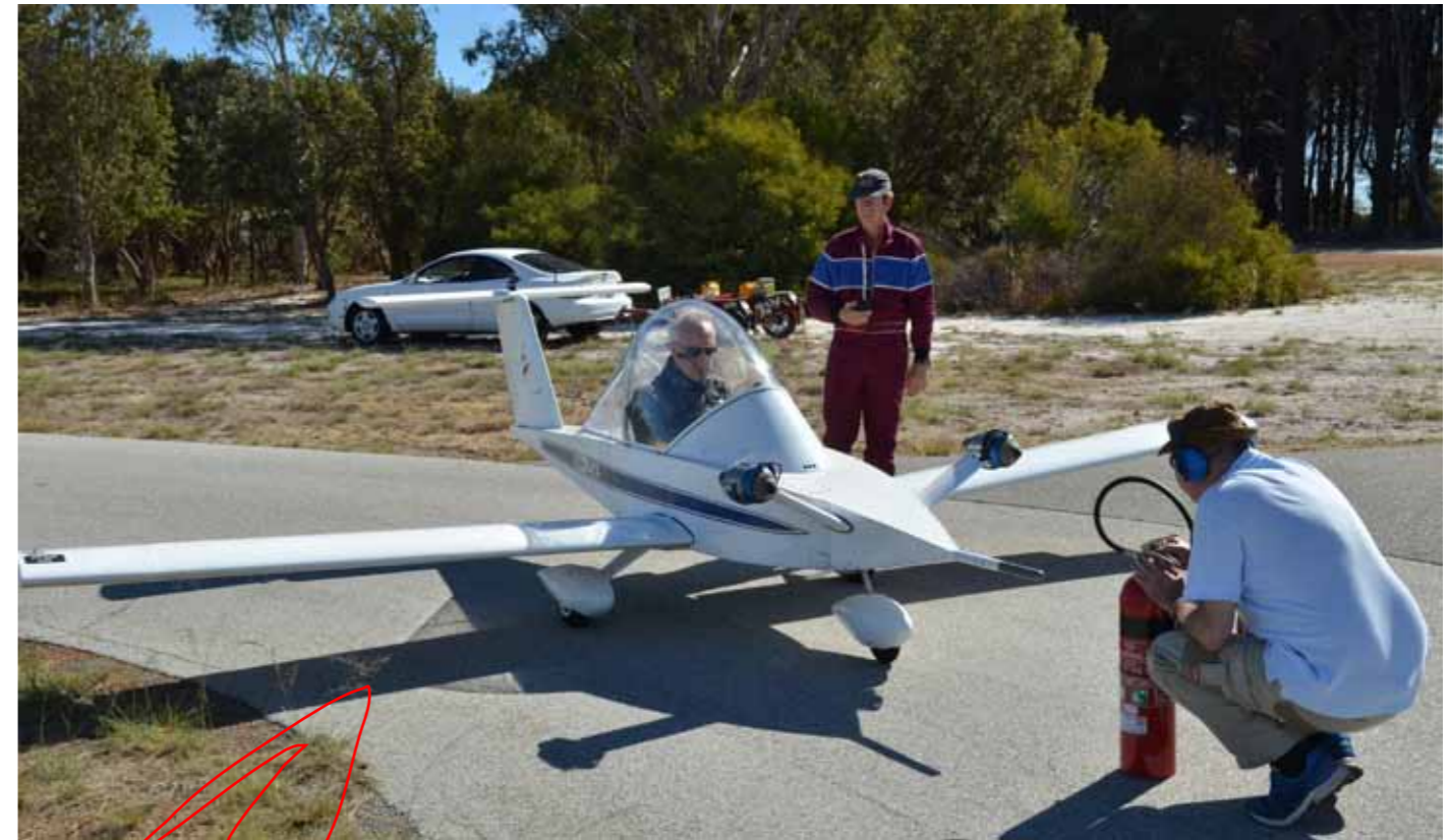
Poised for engine start as close to the runway as practicable to minimise fuel consumed taxiing, ground crew show just how tiny the Cri-Cri is
