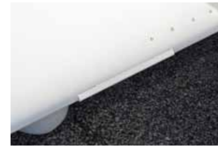
Triangular leading edge strips ('Toblerones') give excellent pre-stall buffet
