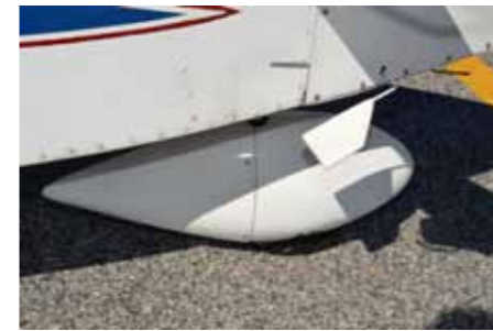
AoA vane sounds a warning horn at 15°, tiny pitot head tube protrudes just ahead of it
