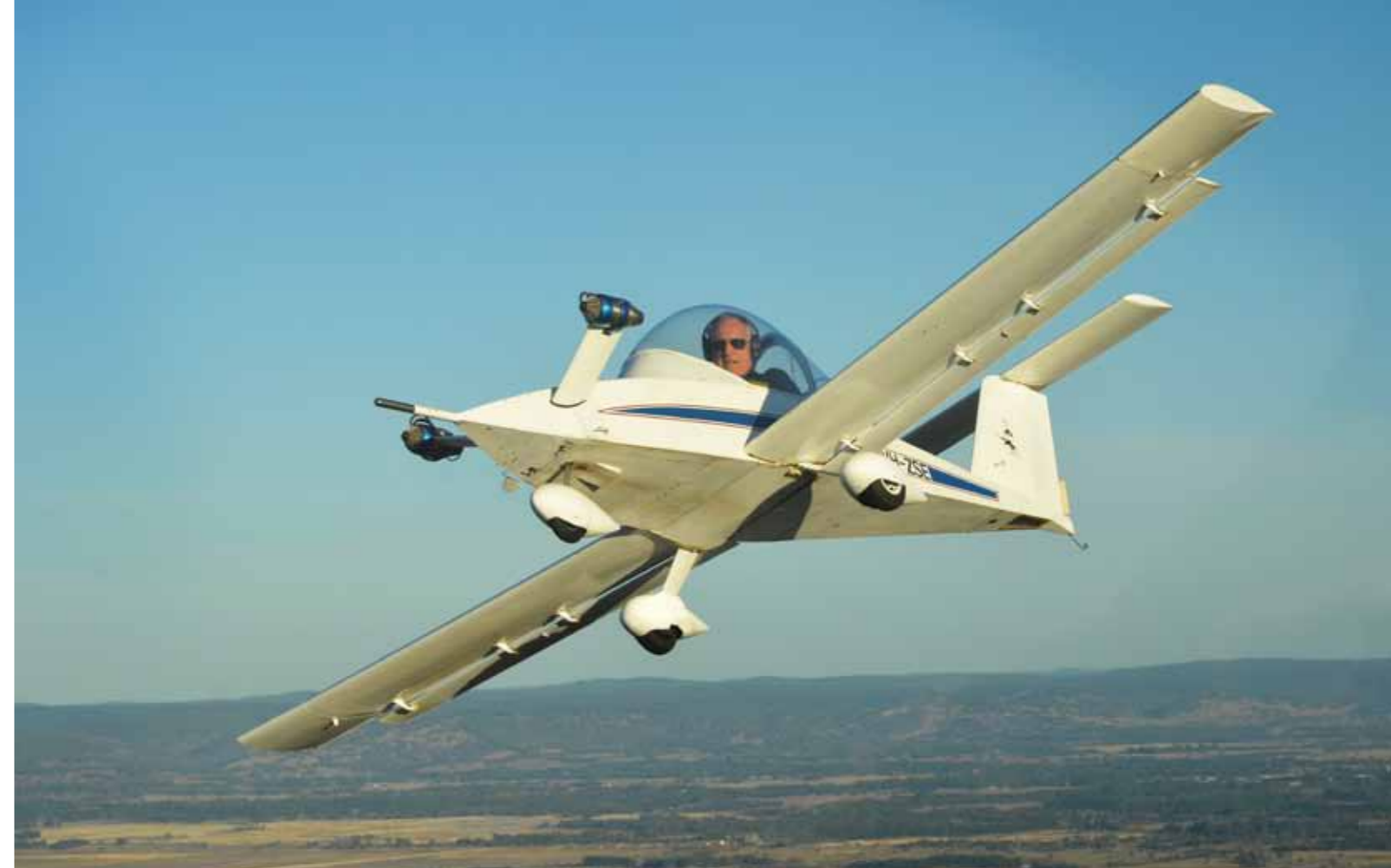
ABOVE: that 'nose probe' is actually a 4.7kg tungsten balance weight on a strong arm, mounted to compensate for the low mass of the turbojet engines
