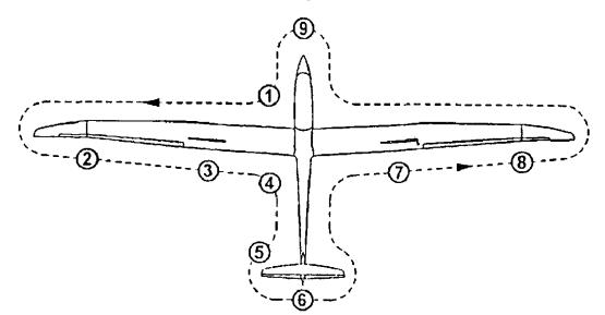
When walking around the "Duo Discus", check all surfaces for paint cracks, dents and unevenness. In case of doubt, ask an expert for his advice.
