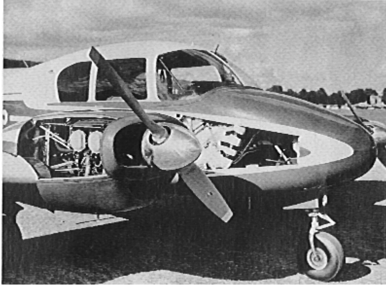
Figure 2 - Photograph of Engine and nose with Panels removed
